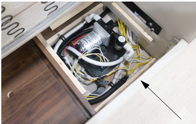
Water Pump (Located beneath sofa seat) -Model 524D shown
