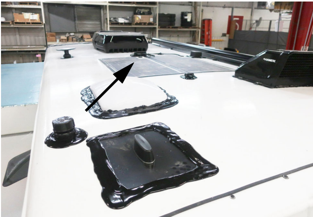
3-Port Solar Cap (Located on the roof) -Typical View
