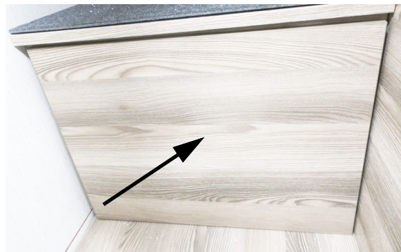
Winterization Valve #1 Pull off the cover to access- located in driver’s side rear closet. On model 524T. -Typical View
