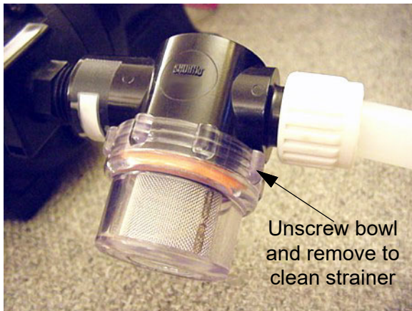
Water Pump Strainer -Typical View
