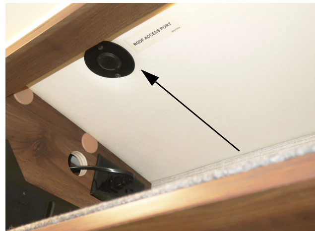
Roof Access Port (Located inside a passenger overhead cabinet) -Typical View
