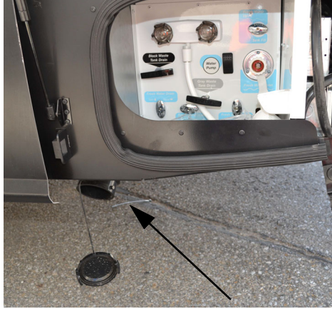
Sewage Drain Outlet Located on the underside of water service center. (524D) -Typical View
