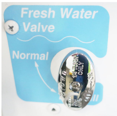
Fresh Water Valve (Located in water service center) -Typical View
